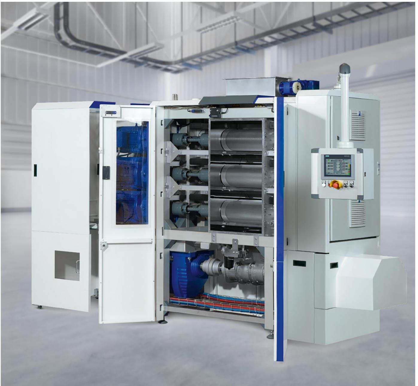
The grinder NEOGRIND has been specially developed to meet sophisticated requirements regarding the control of the grinding particle distribution (PSD) and demonstrates its full grinding efficiency, e.g. for the single cup segment (capsules, pads, etc.). Water cooling of all rollers and the compactor ensures a low temperature level in the grinding process even during intensive grinding.
